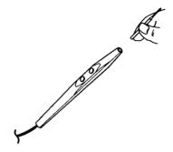
3. Ensure the insulating sleeve fits securely inside the nose of the pencil so that the nose overlaps the insulating sleeve by at least 1/8" (0.3 cm).
